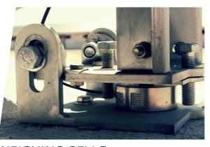
**WEIGHING CELLS** Weighing cells to control consumption.
